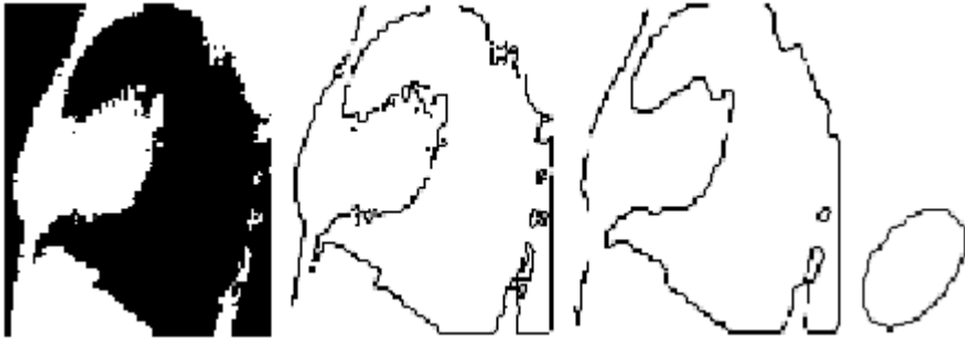
Fig. 6. Lateral Views of image after fuzzy c-means, image with Sobel edge, image with 3*3 structuring element on Sobel edge detected image, and Ellipse found out using curve-fitting method
